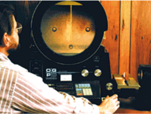
Mechanical specifications are closely inspected with an optical comparator.
