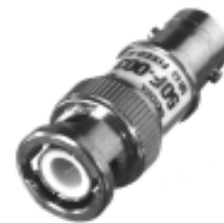
RFA-4050 (3 dB) RFA-4051 (6 dB) RFA-4052 (10 dB) RFA-4053 (20 dB) BNC Attenuator 50 ohm, 1 watt
