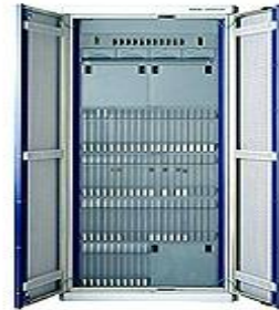
Base Station Controller
