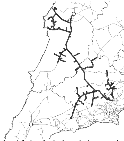
Fig. 7. Evaluated feeder after load transfer between substation (NOP closure and ROSD opening).
