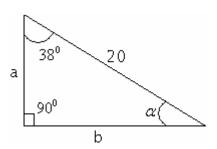
$$\alpha = 180^{\circ} - 90^{\circ} - 38^{\circ} = 52^{\circ}$$
