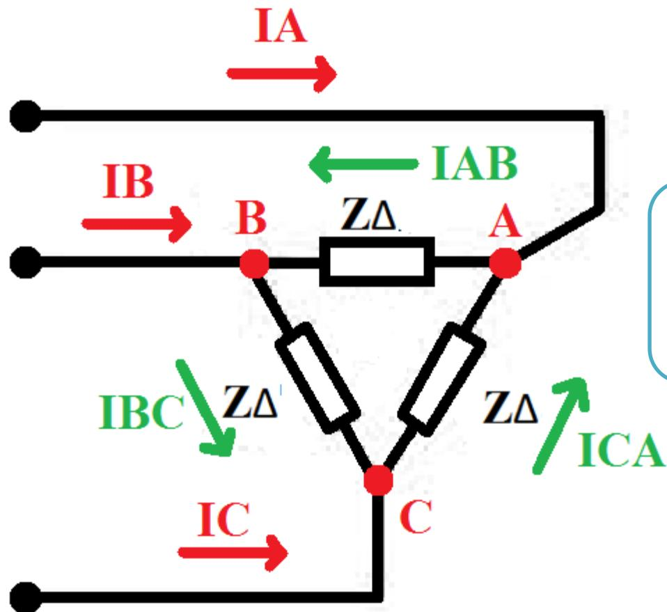
$$I_L = \sqrt{3} I_{PH} \angle -30^\circ \text{ Sec (+)}$$
