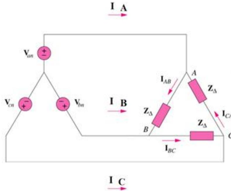
Find  $I_{AB}$  and  $I_B$  if  $V_c = 20 \angle 15^\circ [V]$
