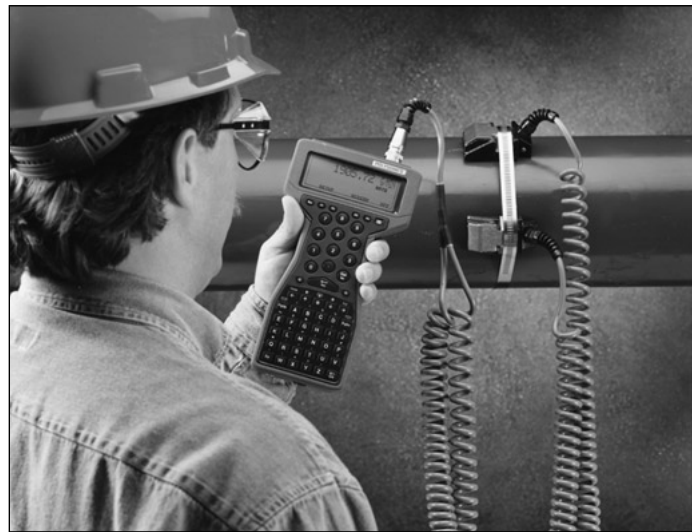
Fig. 6.34 Ultrasonic flowmeters: (a) pulse type; (b) doppler-shift type ( from Ref. 41 ); (c) a portable noninvasive installation ( courtesy of Polysonics Inc., Houston, TX ).
