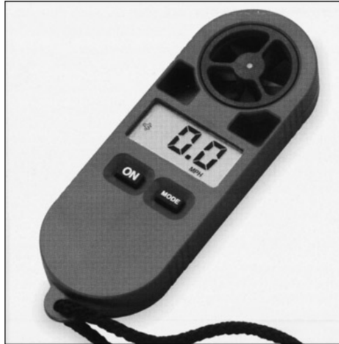
Fig. 6.32 A Commercial handheld wind-velocity turbine meter. (Courtesy of Nielsen-Kellerman Company.)
