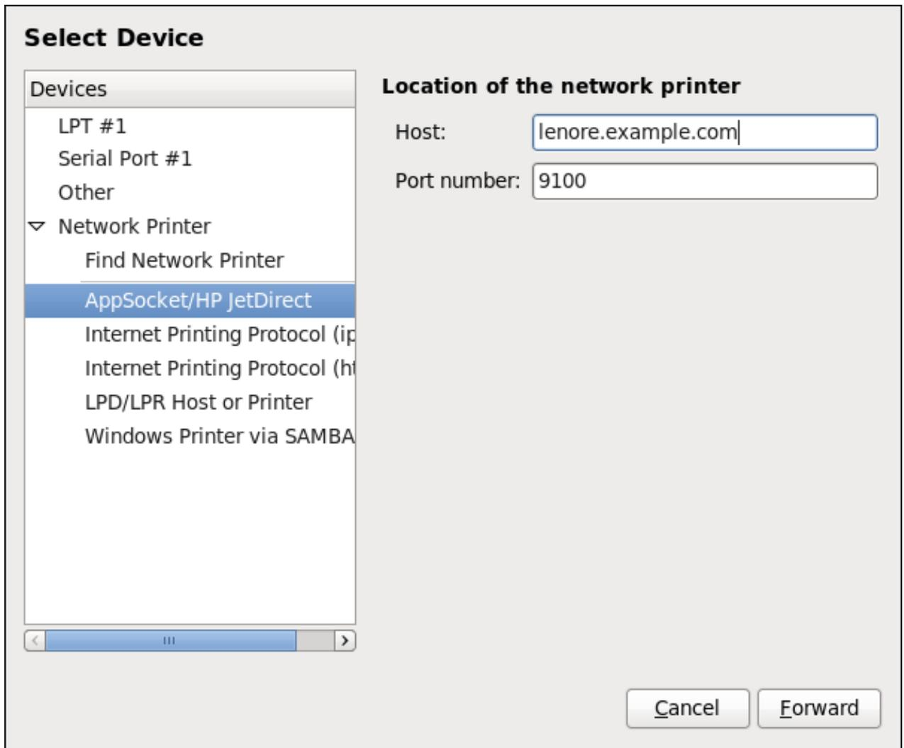
**Figure 14.5. Adding a JetDirect printer**
