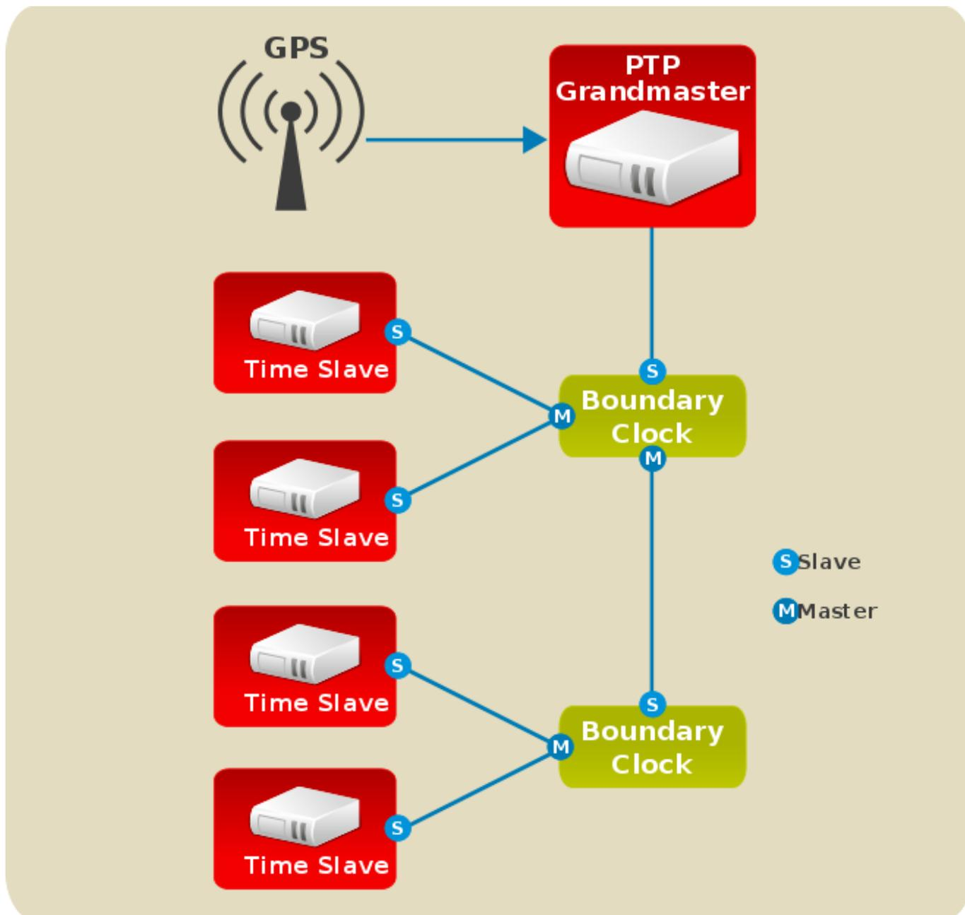
Figure 17.1. PTP grandmaster, boundary, and slave Clocks
