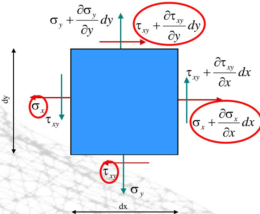
$$-\sigma_x t dy + \left( \sigma_x + \frac{\partial \sigma_x}{\partial x} dx \right) t dy - \tau_{xy} t dx + \left( \tau_{xy} + \frac{\partial \tau_{xy}}{\partial y} dy \right) t dx + b_x t dx dy = 0$$
